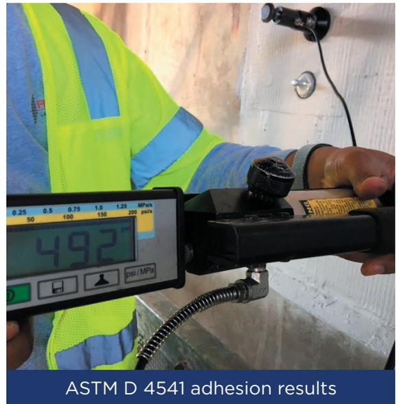
ASTM D 4541 adhesion results
