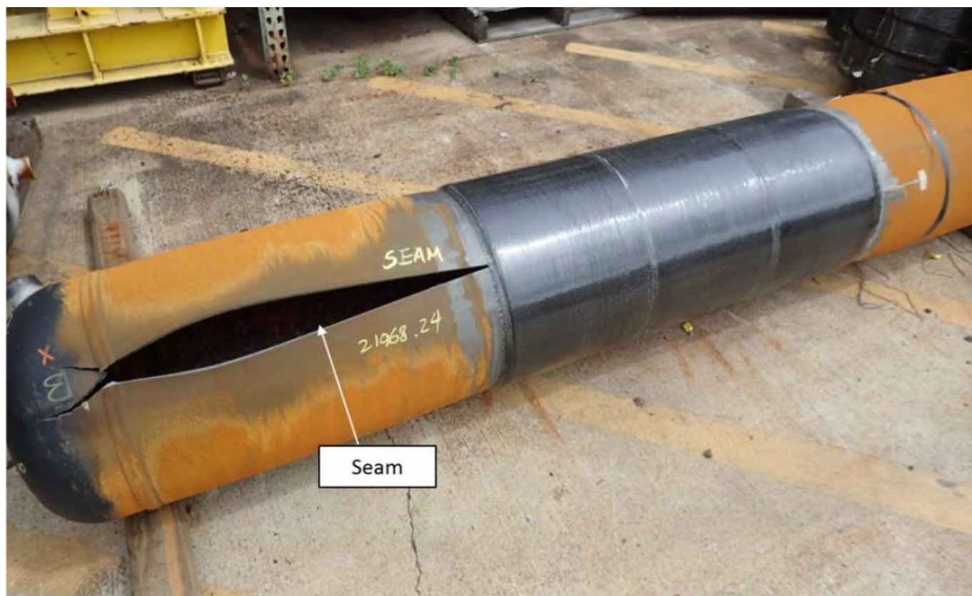
Figure 4. Burst test result of crack repair after cyclic pressure testing.
