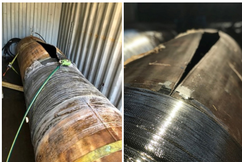
Figure 6. Successful testing with failure outside of the repaired area proved the effectiveness of the Atlas composite repair system.
