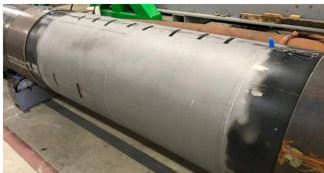
Figure 1. Pipe sample set up for a large-scale bend test to determine the effectiveness of composite repairs for reinforcement in bending such as in geohazard events.
