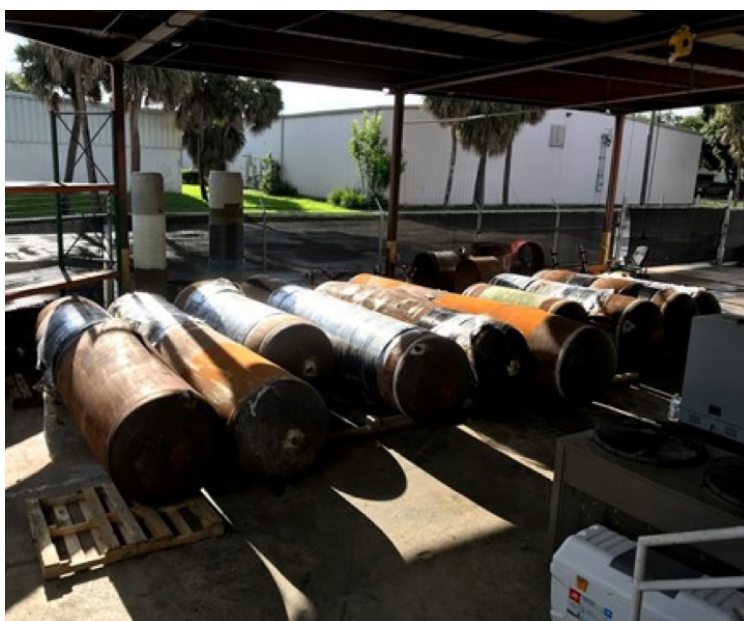
Figure 5. Repaired crack-like defects ready for pressure testing.
