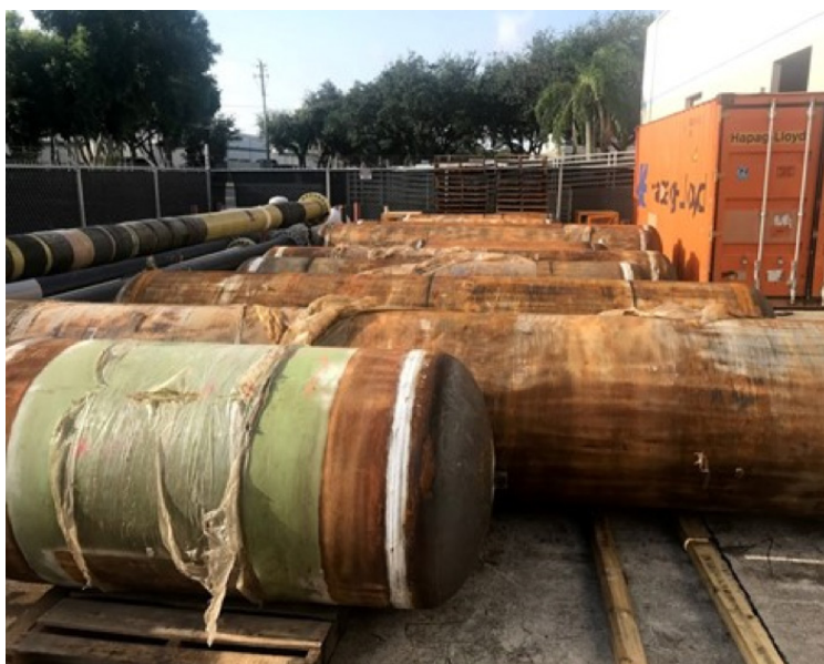
Figure 4. Sections of pipeline with crack-like defects sent to CSNRI for testing.
