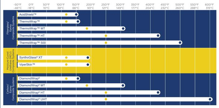
😑 Max recommended installation temp - Exact project parameters may change the recommended temperature.
