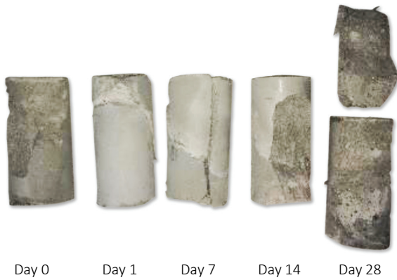
Figure 3. GeoSpray geopolymer slant shear cylinders tested in compression don't have cold joints.
