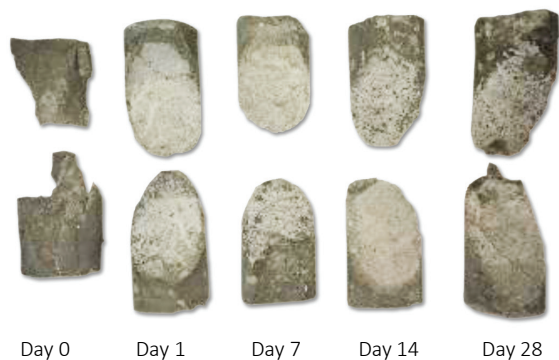
Figure 4. Cylinders of the common pipe rehab OPC product shear on the cold joint in all cases tested.
